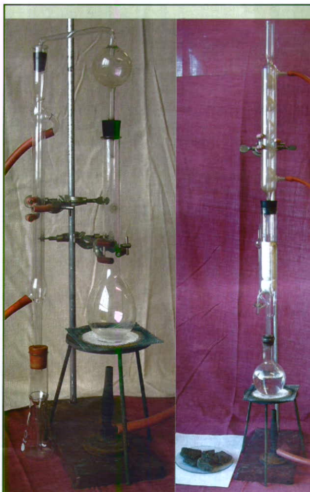
Above: The author's apparatus for (left) Kjeldahl nitrogen determination and (right) Soxhlet extraction with sampling stopcock and filter cake (foreground) ca. 1946 (from L.W. Ruddle).
