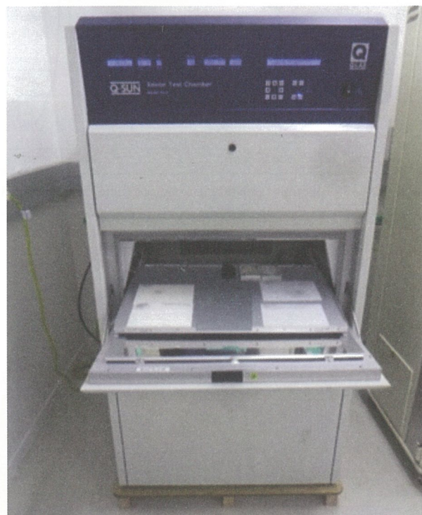
Fig. 2. Polymer specimens in the Q-Sun weatherometer
