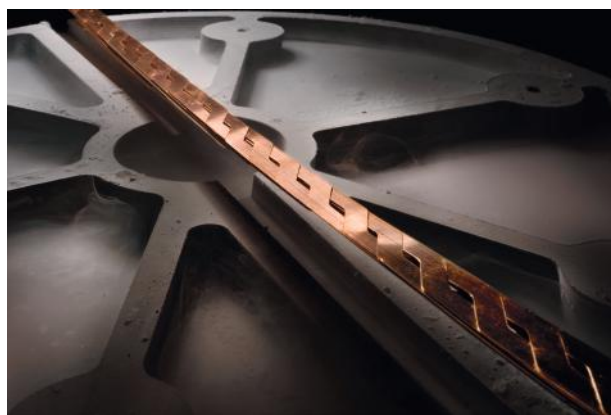
Roebel cable. Photo credit: Robinson Research Institute.
