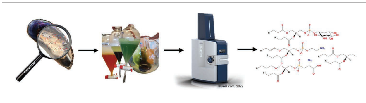
Fig 3. A workflow for phospholipid identification. Left to right: selection of species for study → oil extraction and fractionation → LCMS analysis → phospholipid identification.
